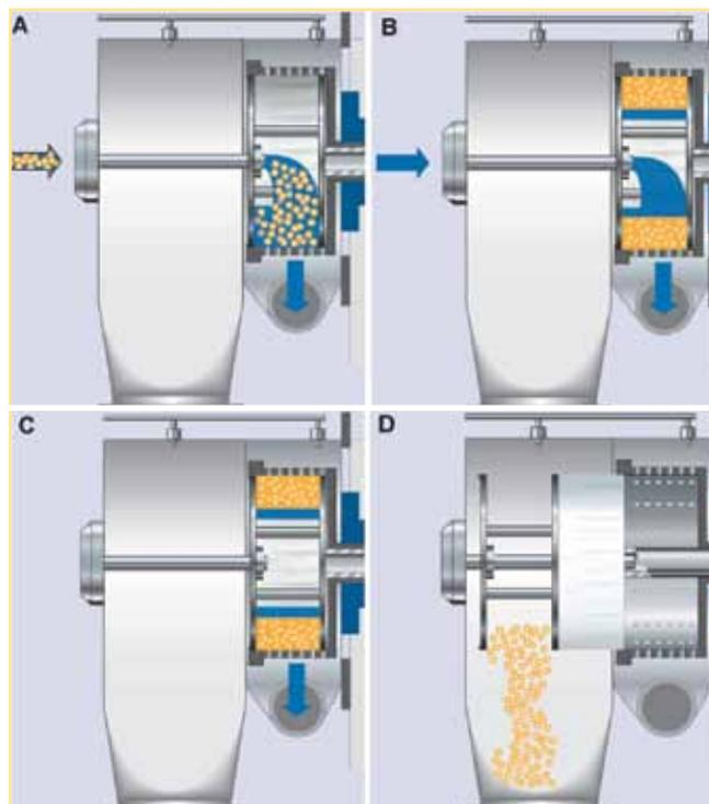
Figure 4. Principal steps of the inverted filter centrifuge a) Filling, b) Washing, c) Drying, d) Unloading.
