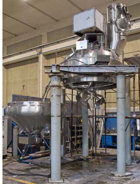
Condry® TDC 3500 dryer with lowered conical bottom
