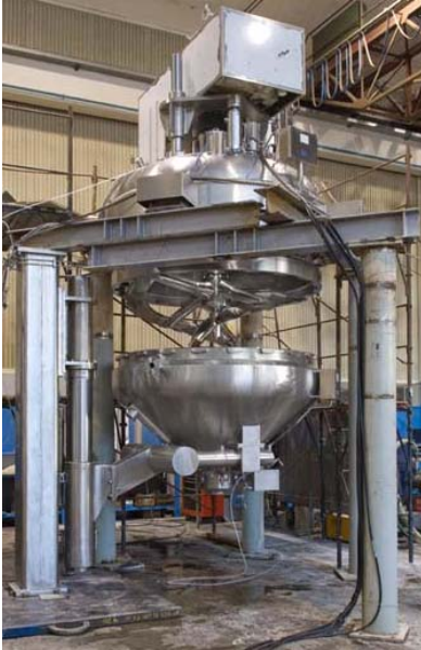
Condry® TDC 3500 dryer with lowered conical bottom
