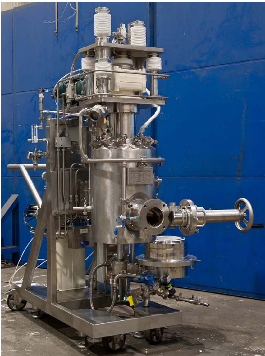
Pressofiltro® PF 10 with 0.045 m 2 filtration area
